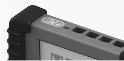
The upper part of the tester accommodates a start button. Press it briefly to start or turn off the instrument. Once the tester has started, a splash screen with a logo will be displayed. Touching the display will bring up the menu. Use the arrows to change the selected option. When the required option is displayed, press the relevant button to select it.
